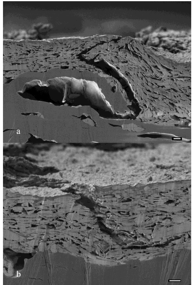
Fig 4. SEM micrographs of coated and creased samples: a) represents clay with 8 pph latex and 8 pph starch, and b) clay with 16 pph latex. The white bars at the bottom right corner of each picture represent 1 \mu\text{m} .
