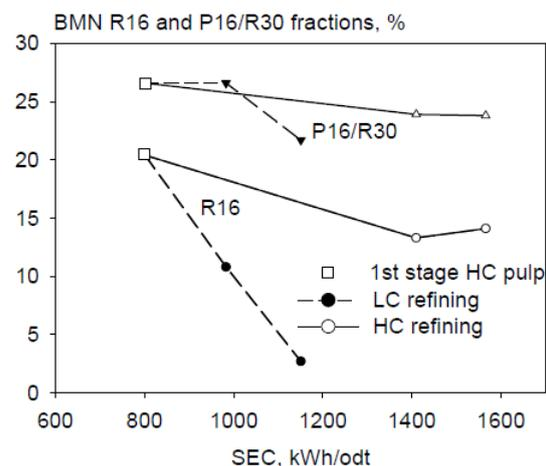
Fig 2. Amount of long fibre fractions (Bauer McNett R16 and P16/R30) in HC and LC refining of primary refined ATMP.
