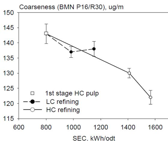
Fig 5. Development of fibre coarseness from HC and LC refining of primary refined ATMP.
