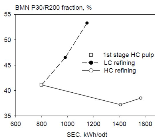
Fig 3. Amount of middle fraction (Bauer McNett P30/R200) in HC and LC refining of primary refined ATMP.
