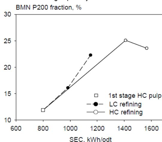
Fig 4. Development of the fines fraction (Bauer McNett P200) in HC and LC refining of primary refined ATMP.
