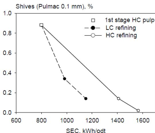
Fig 1. Reduction in Pulmac shives content during HC and LC refining of ATMP with increasing energy input.
