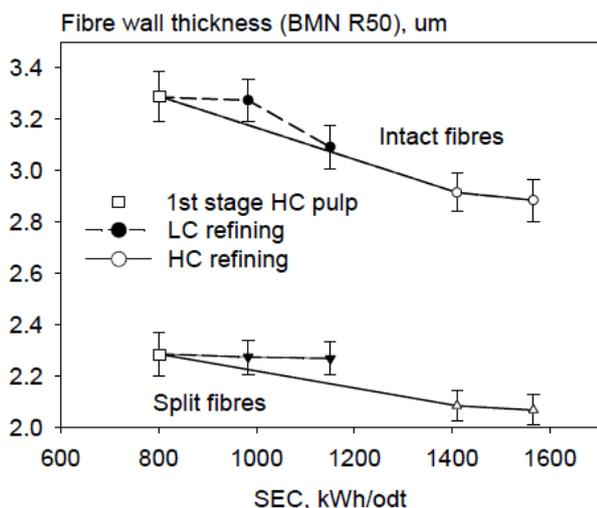
Fig 11. Development of mean fibre wall thickness for intact and split fibre populations in HC and LC refining of ATMP.
