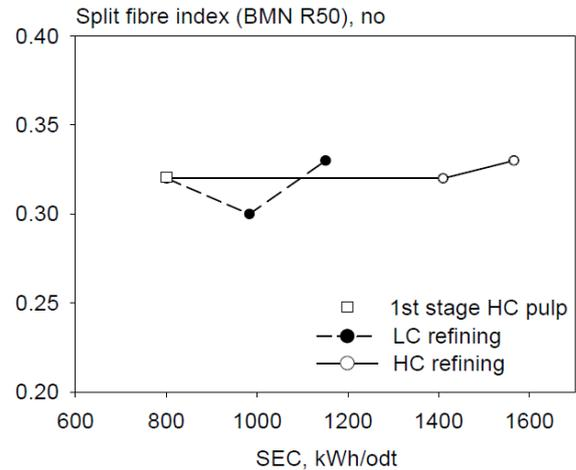
Fig 9. Development of fibre split index in HC and LC refining of ATMP.
