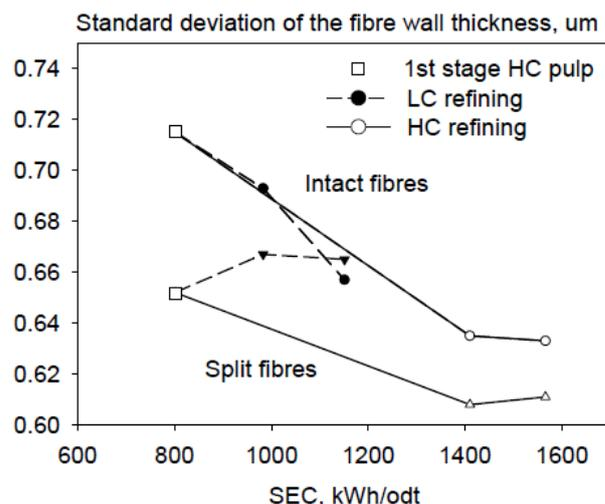
Fig 12. Development of fibre surface homogeneity (expressed as mean standard deviation of the fibre wall thickness) for intact and split fibres from HC and LC refining of ATMP.
