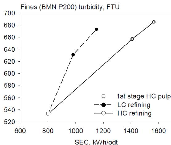
Fig 15. Turbidity of P200 fines formed from HC and LC refining compared at increasing tensile index of handsheets.
