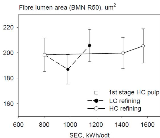
Fig 13. Development of intact fibre lumen area from HC and LC refining of ATMP.
