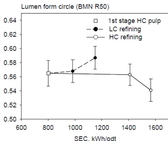
Fig 14. Development of lumen form circle in HC and LC refining of ATMP, intact fibre population BMN R50.
