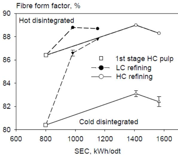
Fig 8. Development of fibre straightness (expressed as fibre form factor) from HC and LC refining of ATMP for hot and cold laboratory disintegrated pulps.
