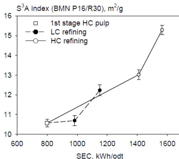
Fig 6. Development of fibre specific surface area (expressed as sedimentation  $S^3A$  index) during HC and LC refining of primary refined ATMP.
