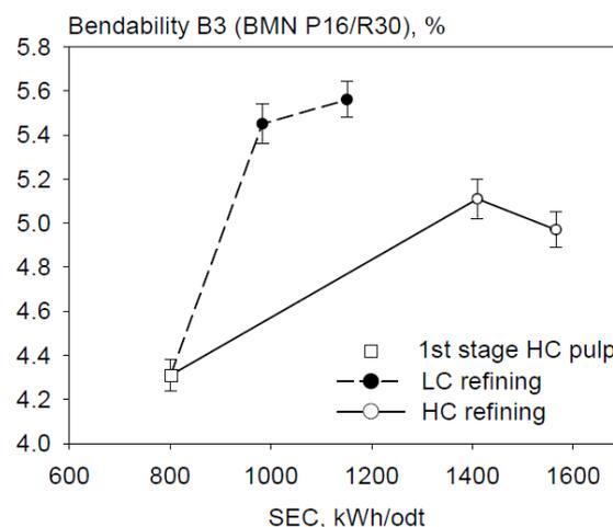
Fig 7. Development of fibre flexibility (expressed as hydrodynamic bendability) in HC and LC refining of ATMP.
