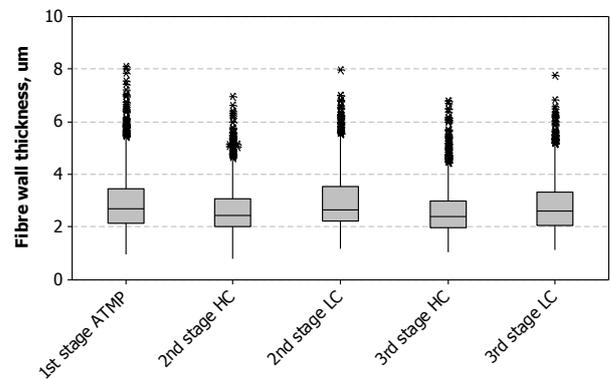
Fig 10. Wall thickness distributions of ATMP fibres before and after two-stage LC and HC Refining (BMN R50).
