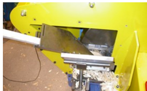
Fig 5. The wood chipper with a sample inserted.
