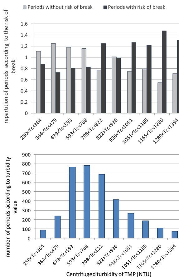
Fig 5. Correlation between turbidity level of TMP pulp and paper web break.
