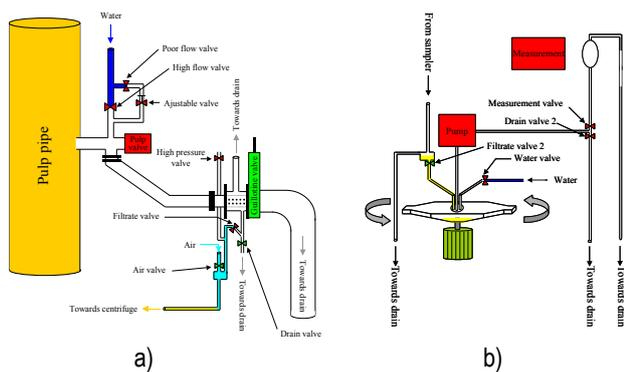
Fig 1. a) schematic blueprint of the sampler
