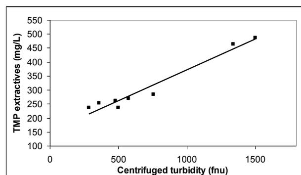
Fig. 4. Extractives level according to centrifuged turbidity of TMP samples
