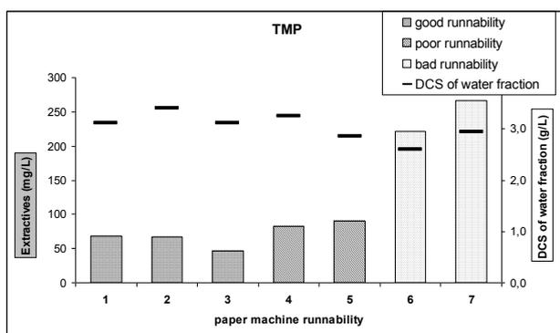
Fig 3. Extractives level according to paper machine runnability.
