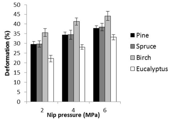
Fig 3. Permanent deformation after pressing as a function of nip pressure.
