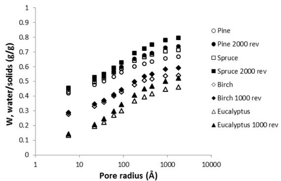
Fig 5. Amount of water (W) as a function of pore radius.
