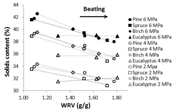
Fig 4. Solids content after pressing as a function of WRV.
