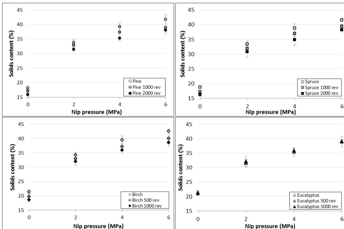
Fig 1. Solids content as a function of nip pressure at different degrees of beating.
