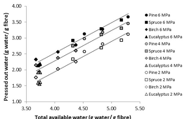
Fig 2. Water removed by pressing as a function of total available water.
